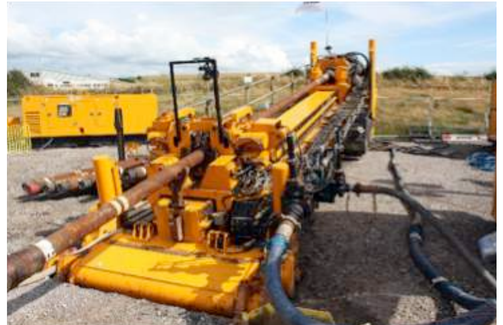
FIGURE 18 IMAGE OF A HDD RIG
